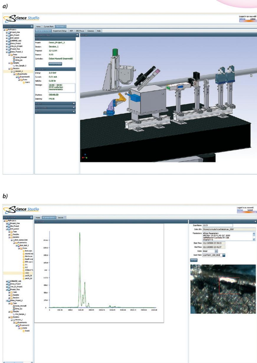
**Figure 1:** Two of the Science Studio screens presently used during a remote XRF experiment are presented here. (a) is the page showing the present beamline conditions (b) the access of data after the experiment, including an optical image of the mapped region and the raw data files that are available for download.
